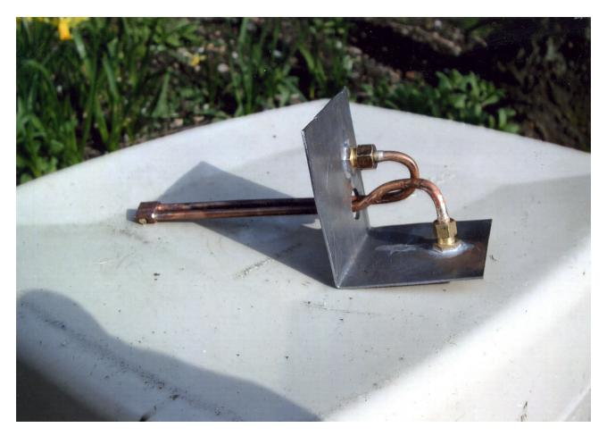
The second picture shows the two parts ready for brazing to the return block. It is worth mentioning that the loco has 2 x 15mm flues instead of the usual nine or eleven at 5/16" diameter. This had worked well on a Gauge One Green Arrow but the shorter ones in this case, cause a fair amount of cinder to be thrown out and the steaming tends to be a little erratic.
