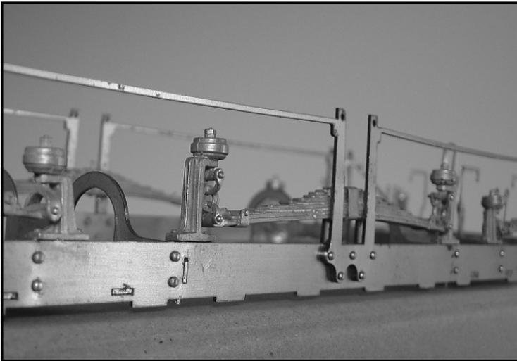
the model has exactly the same, the packing being separate laser-cut pieces.
