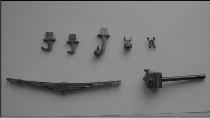
The patterns for some of the brass castings used on the underframe. There are three types of spring hangers, the centre wheels having long "J" hangers and additional links to provide sideplay. On the model these are dummy because the axle is free to slide in and out of the axleboxes. 1mm rivets hold it all together. Including small screws, nuts and rivets, the kit will contain more than
