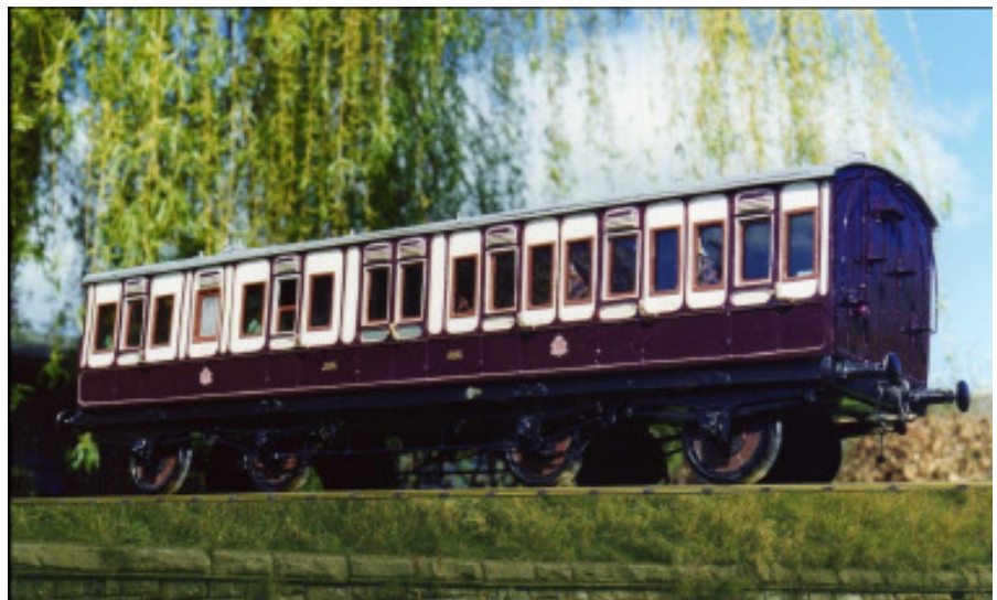
The LNWR six wheeled van has my own variation of the Cleminson flexible under frame. It will go around 4ft radius curves where the eight wheeled composite needs over six foot to run smoothly ! So much for the Webb's patent radial wheelbase on the eight wheeler.
