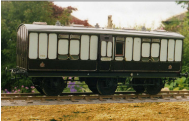
The LNWR six wheeled van has my own variation of the Cleminson flexible under frame. It will go around 4ft radius curves where the eight wheeled composite needs over six foot to run smoothly ! So much for the Webb's patent radial wheelbase on the eight wheeler.
