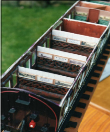
The interior of the third class end of the composite. These had sepia photographs as in the first class end but an advert instead of the mirror. I was able to use reproductions of the old adverts (taken from old magazines) by reducing them on a photocopier. The seating is another moulding in silicone sealant. Third class had boarded floors and no carpets so I only had to paint two for the 'upper class'
