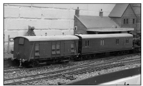
There is a kit of the PLV available and the bogie luggage van can be relatively easily be built from Plastic card, scribed to represent the panelling with roof section as used in the GRS PLV kit. I built my own bogies using shaped steel sides using axle boxes and springs from the PLV kit. bogie The sides are screwed to a pivot block to give a flexible bogie that will ride over most undulations on a garden railway.
